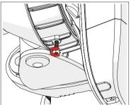
Tighten the locking screw to secure the TwisPort lock mechanism.
