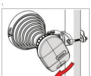
2 Optional: Install the 2.9 x 16mm locking screw.
