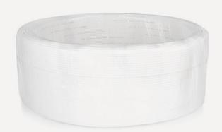
Fiber optic microduct 5/3.5, white (with string) (400m coils) - halogen free microduct, complies with PN-EN 61386-1 standard. Available only in white color. Can be pulled in existing installation ducts or electrical installation pipes. Blowing in and out of fiber optic microcables is fast and easy, so it is possible to replace cables with new ones, to eliminate inactive line or to remove damages.
