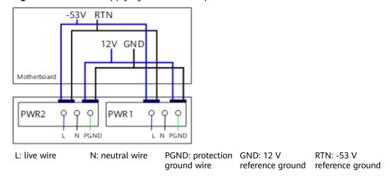
Figure 4-44 Power supply by dual AC PoE power modules
