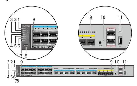
Figure 4-37 Indicators on the S6720-32C-PWH-SI-AC
