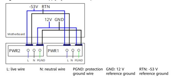
Figure 4-38 Power supply by dual AC PoE power modules
