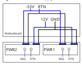
Figure 4-51 Power supply connections of dual DC PoE power modules
