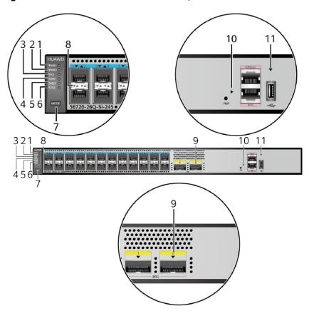
Figure 4-24 Indicators on the S6720-26Q-SI-24S-AC
