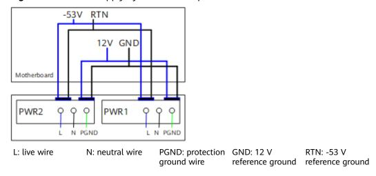
Figure 4-47 Power supply by dual AC PoE power modules
