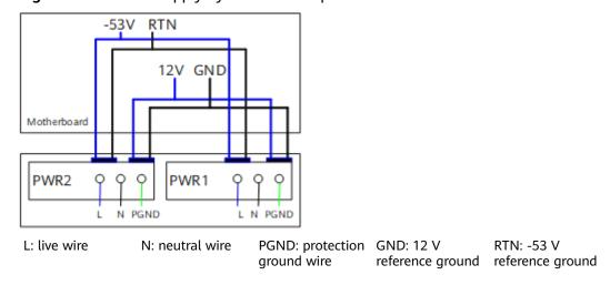
Figure 4-41 Power supply by dual AC PoE power modules
