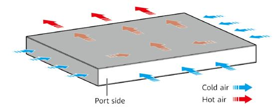
This figure only shows the airflow direction and does not depict the actual device.
