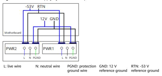
**Figure 4-51** shows the power supply connections of dual DC PoE power modules. After DC power is transmitted to the PWR module, the PWR module provides 12 V and -53 V output voltages, and the motherboard provides 12 V voltage for the entire device and -53 V voltage for the PDs.
