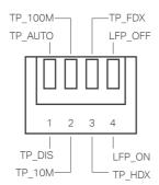
TP\_AUTO/TP\_DIS: Set the TP port speed to Auto-Negotiation/FORCE. TP\_100M/TP\_10M: Set the TP port's speed. LFP\_ON/LFP\_OFF: Enable or disable the LFP function. TP\_FDX/TP\_HDX: Set the duplex mode for the TP port as Full-Duplex/Half-Duplex.
