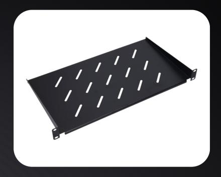
Fixed shelves are manufactured in standard depths from 250 to 750 mm and in height 1U. Fixed shelves are designed for mounting in a 19" rails in 2 points on the front or the back of the bar.
