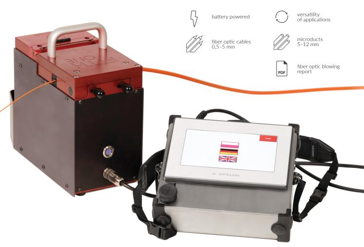
The **FTTH One** blowing machine is the perfect solution for blowing the thinnest optical fibers due to fully adjustable feeding speed and feeding force. Magnetic clutch and precisely selected blowing parameters protect the cable against damage.
