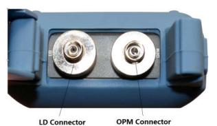
**LD Connector:** Light Source output interface (When the light is turned on, please don't look directly into optical output or connected fiber optic connectors, in order not to
