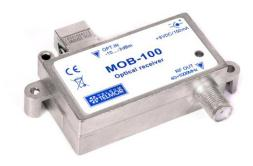
Micro optical receivers MOB-100 are the modern devices dedicated for FTTH (*Fiber To The Home*) applications. This device is made in die-cast metal housing and can be mounted in plastic housing "mouse" type. Receiver is equipped with SC/APC input connector and one RF output with "F" female connector. Optical receiver is also equipped with LED 3-stage optical input power indicator.
