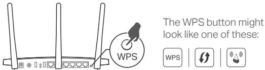
2. Within 2 minutes, press the button on the extender for 1 second.
