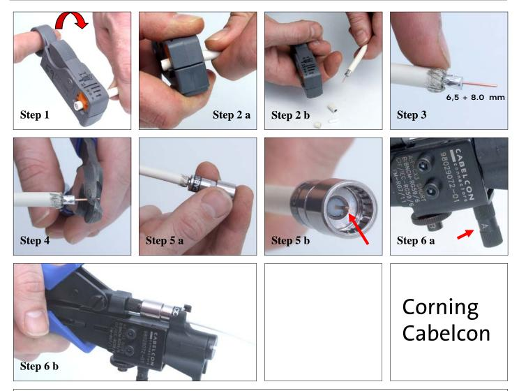
STEP 1: Insert the cable as shown. Turn the tool clockwise 5-7 times.
