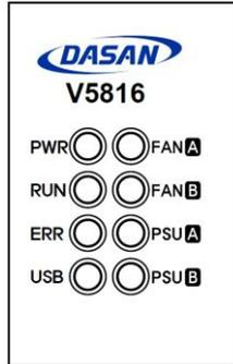
**Figure 3** LEDs of Power System & FAN
