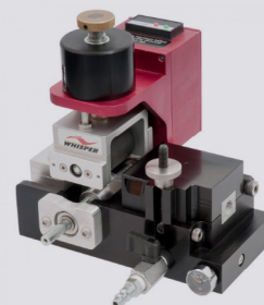
Whisper Microcables/cables 3-8,5 mm microducts 4-18 mm
